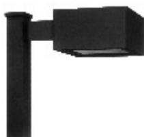
**GOOD** Flat-lens shoebox fixtures come in many forms; square, rectangular, circular, etc. All control the light with internal reflectors. Glare and light trespass are minimized; no uplight is produced.
