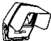
**GOOD** If floodlights must be used, they should always have top and side shielding, and be pointed at least 45 ° below the horizontal.
